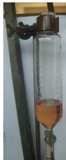
Figure 3. Fuel consumption measurement: (a) connection of the measuring vessel to the engine; (b) measuring vessel.
