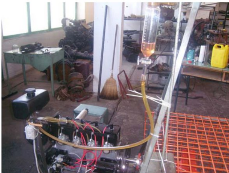
Figure 3. Fuel consumption measurement: (a) connection of the measuring vessel to the engine; (b) measuring vessel.
